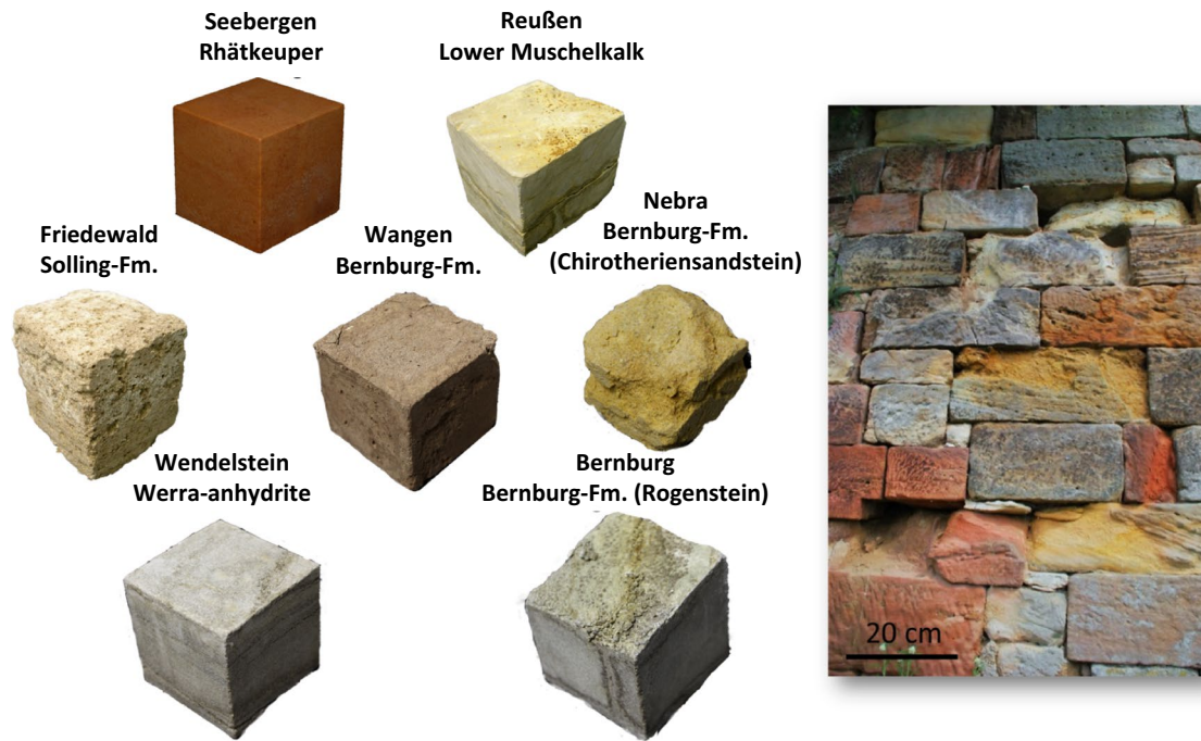
Fig. 4 Analysis of weathering phenomena. Left: artificially weathered building stone samples subjected to “salt splitting tests” by several cycles of soaking with sodium sulfate solution and subsequent drying. As also documented for stones in a wall section (right), resist-
