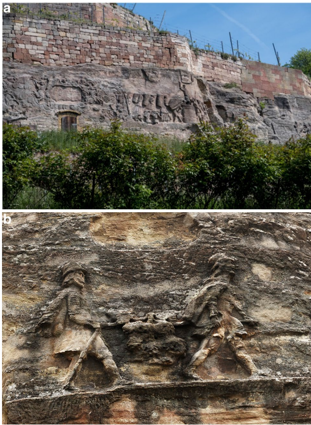
Fig. 5 The “Stone Album” (near Großjena) showing various weathering phenomena on the outcropping rock (Middle Buntsandstein). a overview, b small, heavily weathered section
